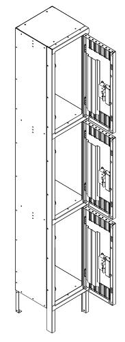
**10.** Anchor units to wall or floor. The units are not intended to stand free and may topple if not secured. Units standing back to back should be bolted back to back.
