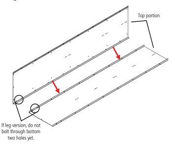
**5.** Bolt the right side (Ref. No. 6) to the back so that the side flange fits around the back also attaching to the top, middle and bottom shelves using twenty-two nuts and bolts if the locker has no legs and twenty-four nuts and bolts for a locker with legs. Attach the remaining hooks to the right side over the flange of the shelves using two nuts and bolts on each hook.
