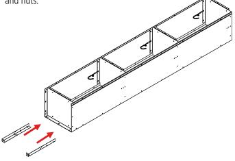
**7.** Place the door and frame assembly (Ref. No. 7) over the locker body. Make certain that body sides are inside frames.
