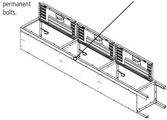
**9.** Stand the unit upright and place in the desired location. Remove temporary bolts in frames and bolt to adjacent units together through frames.
