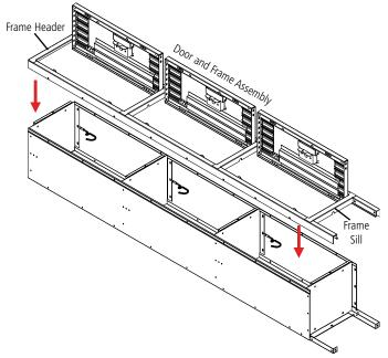
**8.** If joining units side by side, temporarily install only one bolt and nut in the frame(s) that will be joined to the adjacent locker frame(s). If locker is just a single unit, finish attaching the frame using twenty bolts and nuts. Check and tighten all
